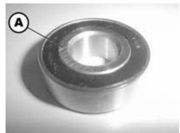
The steering wheels should always rotate freely after mounting, but the bearings may not have any play.
