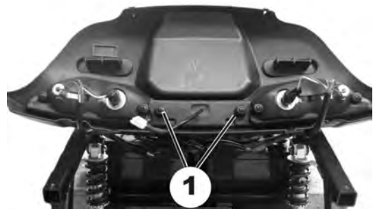
Remove screws (1) on brake light.
