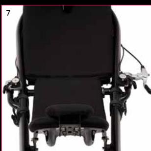
7. Options for cyclists with limited hand function are the Double Tap Frame Mounted Shifters which are positioned so that the right shifter operates lower derailleur and the left operates upper chainrings by using your elbows. Add the Elbow Activated Frame Mounted Brake and you are good to stop and go! A disk brake is recommended for added safety and "stoppability."
