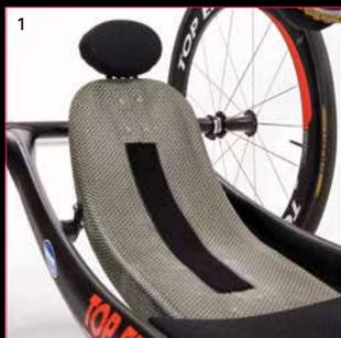
1. The totally adjustable featherweight carbon fiber back is as lightweight as the fixed welded back, allowing athletes the ability to find their most aerodynamic and powerful position for the course, whether it is a road race, time trial or triathlon.
