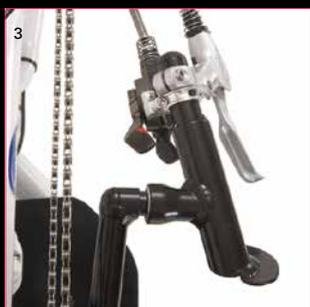
3. The SRAM® X9 30 speed drive train, trigger shifter and brake mounted on the right handpedal is standard. This allows for hands-on shifting and braking right at your fingertips.
