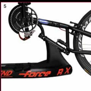
5. The redesigned curved monocoque front triangle is super strong and looks terrific. This new design allows the athlete to get closer to the front wheel which translates to a lighter and stiffer fork because it is shorter. Plus, it allows for more body clearance so the athlete can get lower and obtain a more streamlined position.
